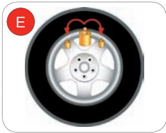
**(EN) HIDDEN WEIGHT AND SHIFT PLANE PROGRAMS (ALU P):** «Hidden Weight» subdivides the external adhesive weight in 2 parts to be positioned behind the spokes of the rim. The patented program «Shift Plane» calculates the balancing position to allow using commercial adhesive weights.
