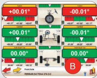
**(EN) ALIGNMENT SOFTWARE:** Professional alignment software complete with an easy-to-use and intuitive user interface to prevent operators from making errors during the different working phases. Possibility to customize display, key functions and languages.
