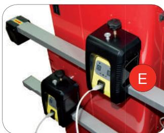
**(EN) POWER SUPPLY SYSTEM:** Power supply system by means of commercially available type AA rechargeable batteries with recharger device integrated on cabinet. Emergency cables are also available on demand.
