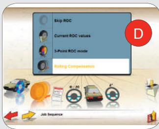
**(EN) «RUN-OUT» COMPENSATION PROGRAMS:** Available 2 different programs to compensate «Run-Out» problems and possible mistakes caused by an incorrect coupling between rim and clamp: 3-point ROC by rotating the clamp of 180° and push mode ROC which eliminates the need to lift the vehicle.
