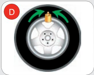
**(EN) AUTOMATIC BALANCING POSITION SEARCH:** Lowering the wheel cover, the shaft starts to rotate thus activating the balancing cycle. After the spin, the TECO 710 automatically stops the wheel at the right weight application position, both for internal and external side of the rim.
