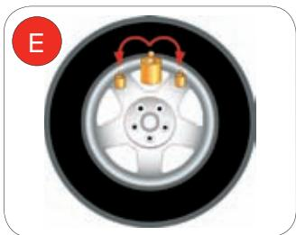
**(EN) HIDDEN WEIGHT AND SHIFT PLANE PROGRAMS (ALU P):** «Hidden Weight» subdivides the external adhesive weight in 2 parts to be positioned behind the spokes of the rim. The program «Shift Plane» calculates the balancing position to allow using commercial adhesive weights.
