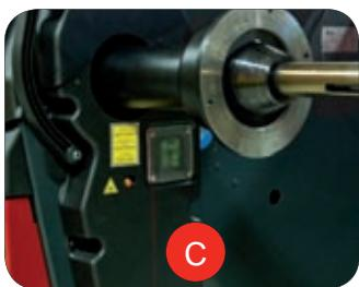
**(EN) LASER LINE AND RIM ILLUMINATOR:** Standard with Laser line system and rim illuminator. If ALU programs are selected, the Laser line assists the operator during adhesive weight positioning at 6 o'clock. The rim illuminator supports operators during rim cleaning and weight application.
